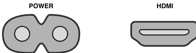
Figure 1.4 The sockets on the back of a TV are deliberately different shapes to make it hard to plug the wrong cables into the wrong holes.
