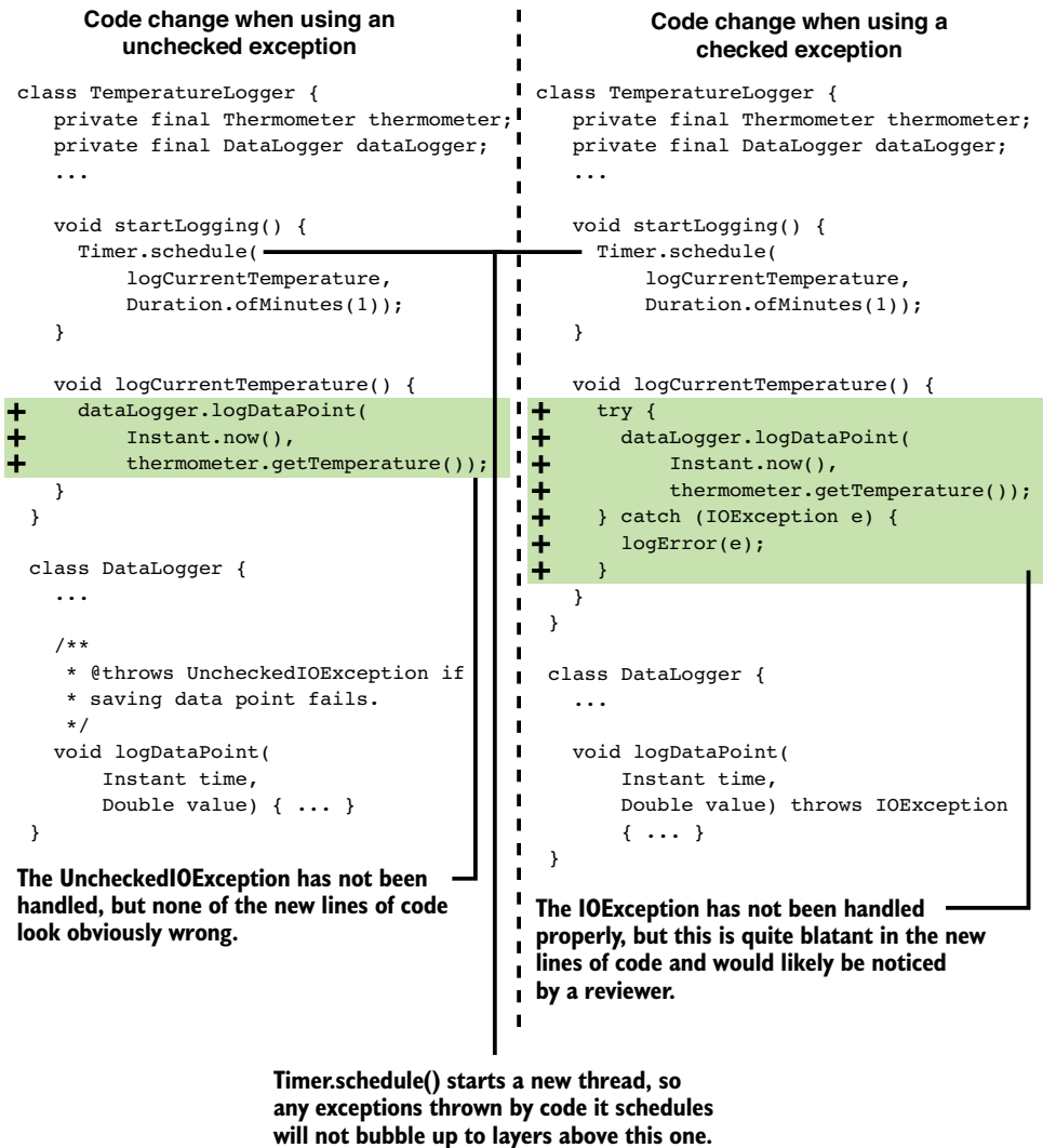
Figure 4.5 When using explicit error-signaling techniques, not handling an error properly will often result in a deliberate and blatant transgression in the code. By contrast, when using an unchecked exception, it may not be obvious from the code that an error has not been handled properly.
